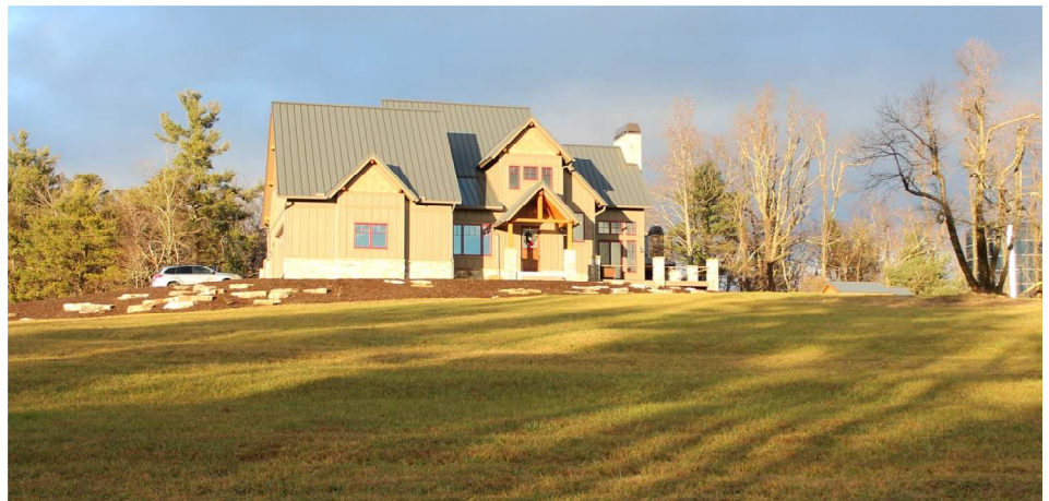
The Freeman-Rash home is also an example of "firewise" landscaping because it has at least a 50 foot grass and mulch/rock perimeter around the house with few trees or downed dead fuels.
